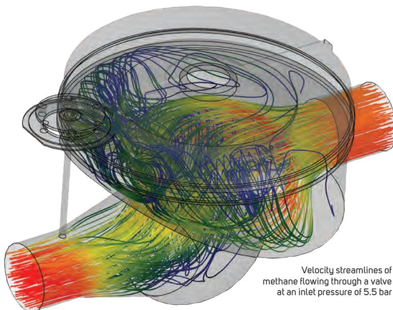
Velocity streamlines of methane flowing through a valve at an inlet pressure of 5.5 bar
